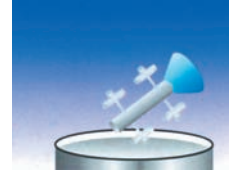
4. Dipping into ceramic slurry
